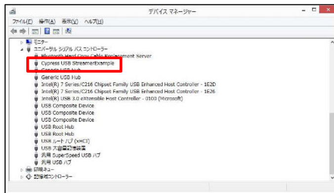
Figure 1 Check device driver
