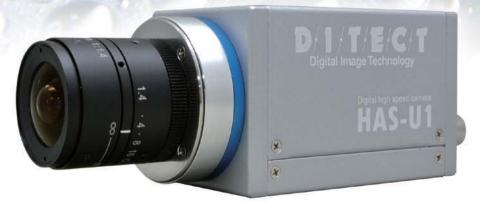
HAS-U1 is a high speed camera with ½-inch CMOS sensor and 1. 3M 1280 × 1024 effective pixels that can shoot 200 fps at full resolution, 800 fps at VGA, and up to 4,000 fps by limiting the pixel area. Perfect for multiple high speed camera imaging, with embedded memory, in one compact solution.
