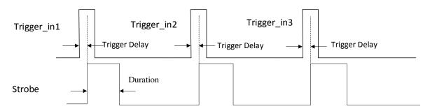
Figure 9-7 Sequence Diagram of Strobe Line Duration
