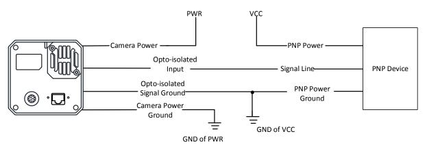
Figure 10-9 Input Signal Connects to PNP Device
