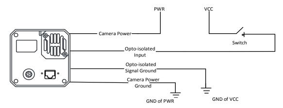
Figure 10-11 Input Signal Connects to Switch
