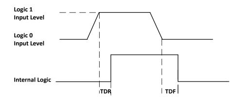
Figure 10-2 Input Logic Level
