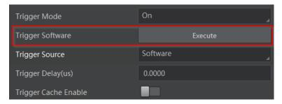
Figure 8-8 Set and Execute Software Trigger
