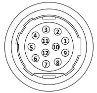
Figure 3-2 12-Pin P10 Connector
