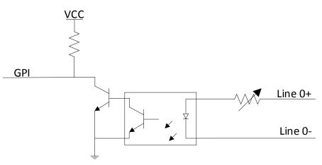
Figure 10-1 Internal Circuit of Input Signal
