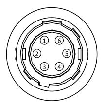
Figure 3-1 6-Pin P7 Connector
