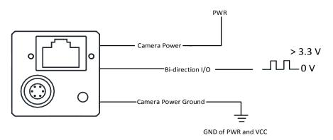
Figure 10-16 Input Signal Connects to Switch
