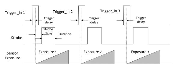
Figure 9-9 Sequence Diagram of Strobe Line Delay
