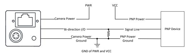
Figure 10-14 Input Signal Connects to PNP Device
