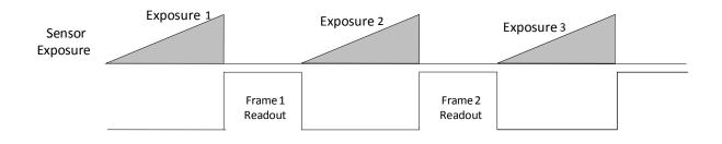
Figure 7-5 Internal Trigger Non-Overlap Exposure
