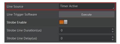
**Figure 9-4 Timer Active Parameters**
