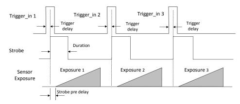
Figure 9-11 Sequence Diagram of Strobe Pre Line Delay
