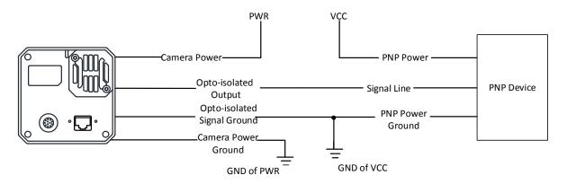
Figure 10-12 Output Signal Connects to PNP Device
