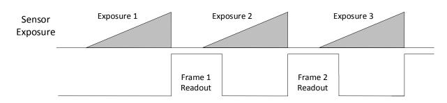
Figure 7-7 Internal Trigger Overlap Exposure
