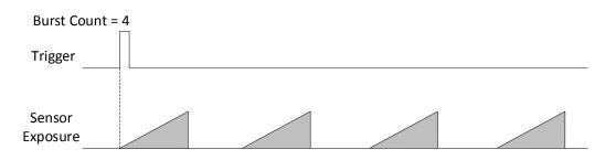
Figure 8-16 Sequence Diagram of Acquisition Burst Frame Count
