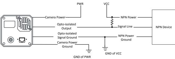
Figure 10-13 Output Signal Connects to NPN Device
