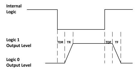
Figure 10-8 Output Logic Level
