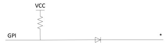
Figure 10-5 Internal Circuit of Non-Isolated Input
