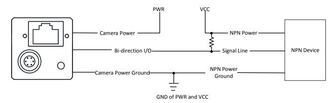
Figure 10-18 Output Signal Connects to NPN Device
