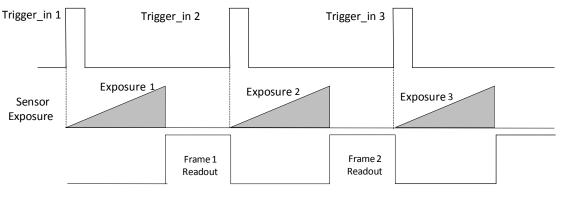
Figure 7-6 External Trigger Non-Overlap Exposure
