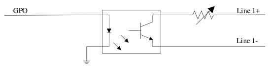
Figure 10-3 Internal Circuit of Output Signal
