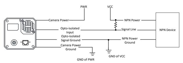
Figure 10-10 Input Signal Connects to NPN Device
