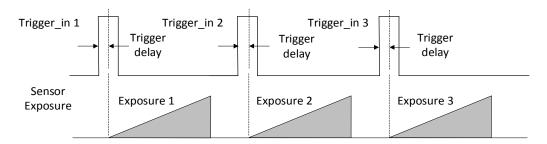
Figure 8-19 Sequence Diagram of Trigger Delay
