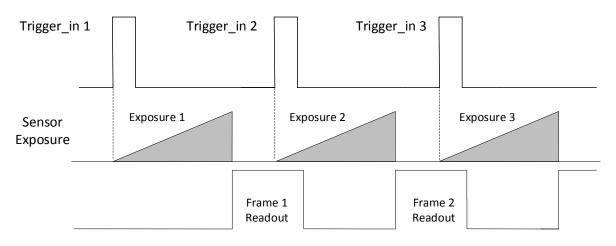
Figure 7-8 External Trigger Overlap Exposure
