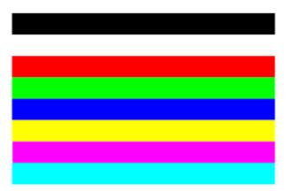
Figure 11-19 Horizontal Color Bar Test Pattern
